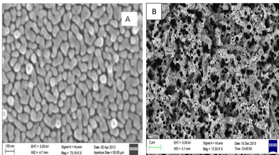
**Figure 2.** SEM images of (a) Silver nanoparticle (AgNP) deposition (b) pores on silicon after dissolution of Silver (Ag).
