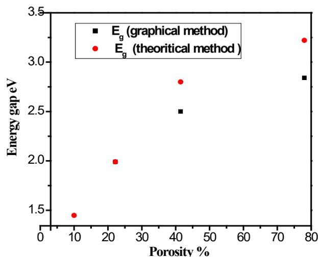
Figure 7. Variation of optical energy gap with porosity.
