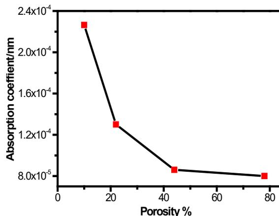
**Figure 5.** Variation of absorption coefficient with porosity.
