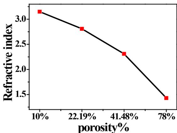
**Figure 4.** Variation of refractive index of PS with porosity.
