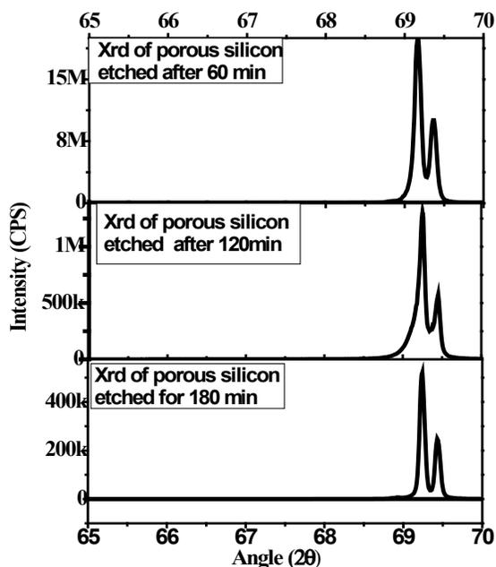
**Figure 1.** XRD patterns of porous silicon fabricated at different etching times.
