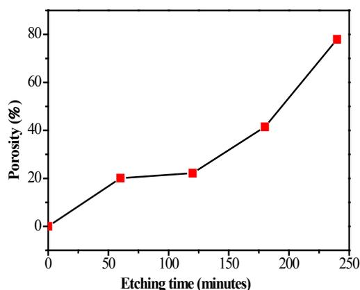
Figure 3. Variation of porosity with etching time.
