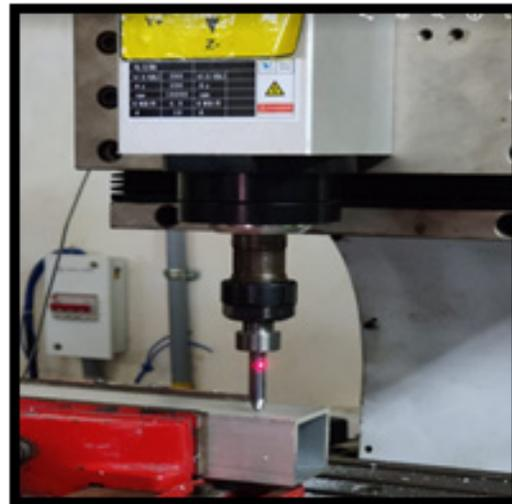
**Figure 4.** Experimental Setup for friction drilling.
