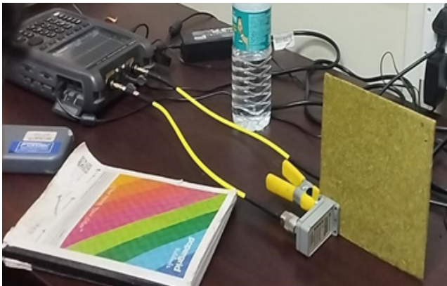
Figure 3. Electromagnetic shielding effectiveness experimental setup
