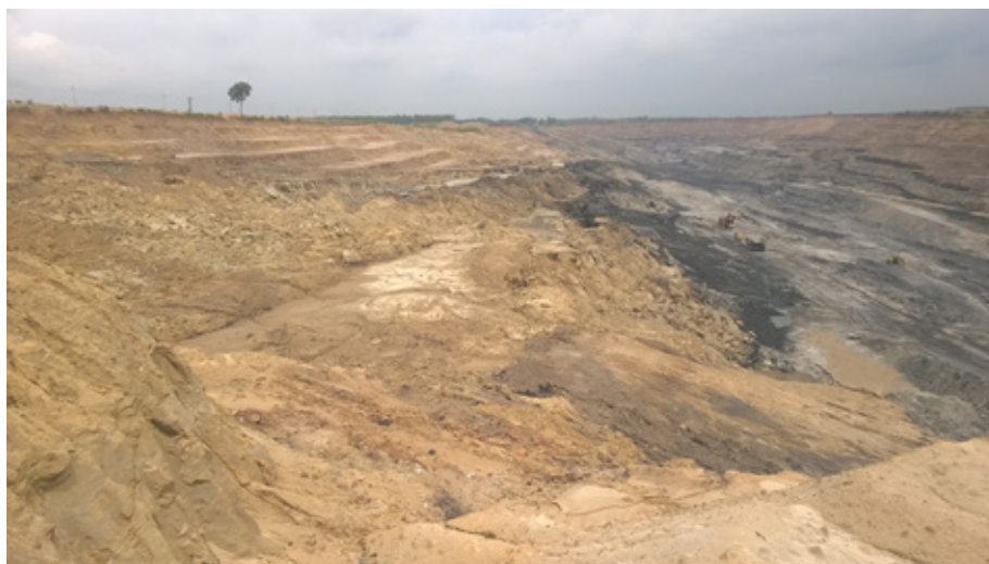
Figure 1. A view of the rise side highwall slope of OC mine.
