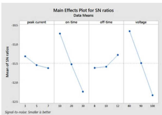
**Figure 2a.** Main effect plot of average roughness.
