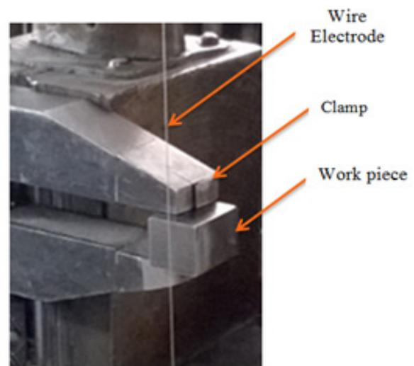
Figure 1a. Machining arrangement.
