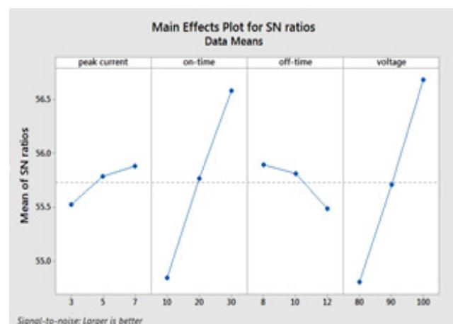
**Figure 2b.** Main effect plot of material removal rate.
