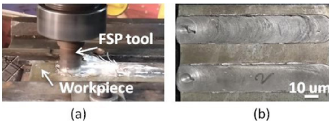
Figure 2. Photograph showing FSP of WE43 Mg alloy.
