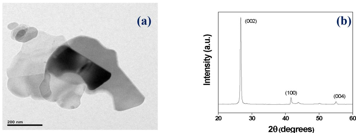
**Figure 1.** (a) TEM and (b) XRD of hBN nanoplatelets.
