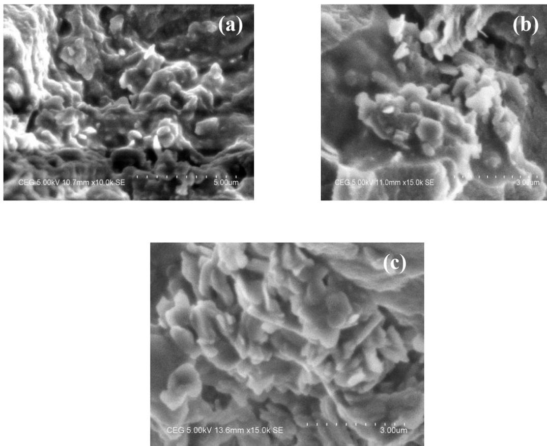
**Figure 2.** SEM images of (a) PSS+1 wt.% hBN (b) PSS + 3 wt.% hBN(c) PSS + 4 wt.% hBN nanoplatelets.
