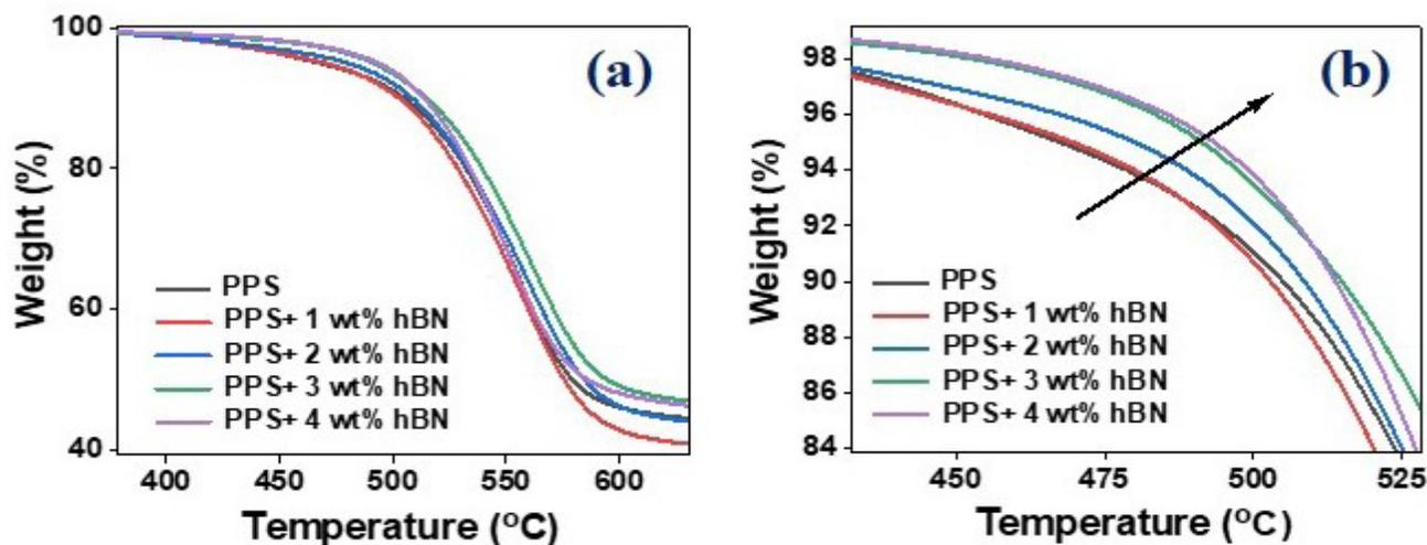
Figure 4. TG curves of PPS and hBN nanoplatelets filled PPS nanocomposites.
