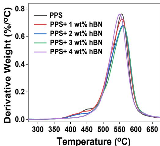
Figure 5. DTG curves of hBN nanoplatelets filled PPS nanocomposites.
