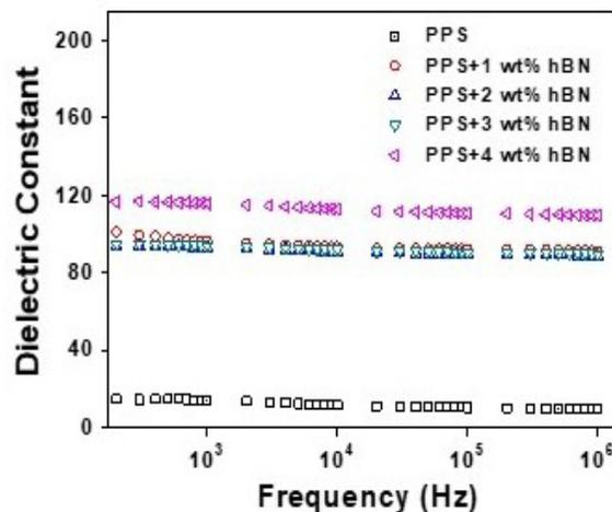
Figure 6. Dielectric constant of hBN filled PPS nanocomposites.
