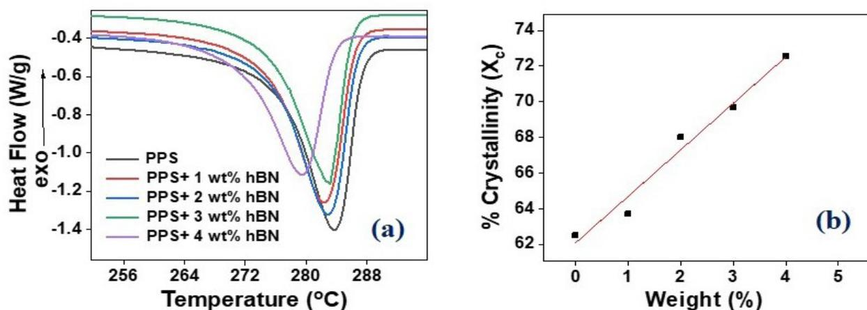
**Figure 3.** (a) Melting endotherms (b) % Crystallinity of PPS and hBN nanoplatelets filled PPS nanocomposites.
