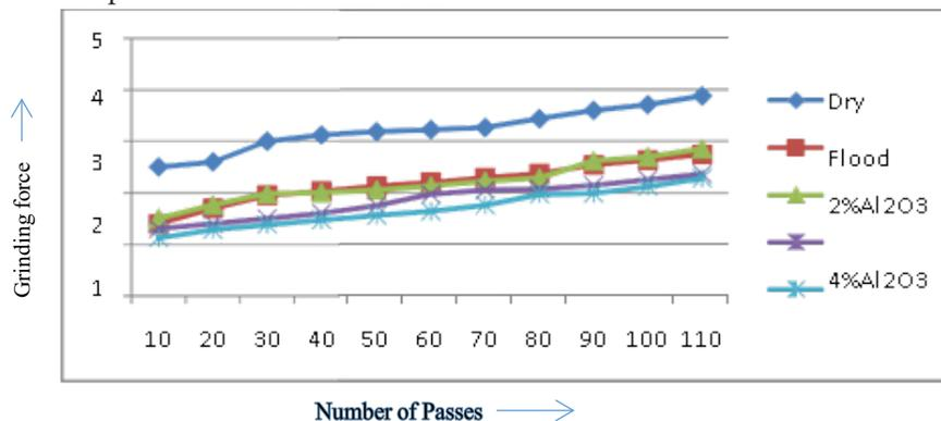
Figure 5. Specific Tangential grinding force vs number of passes.
