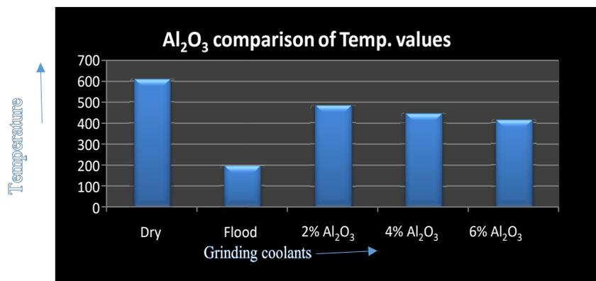
Figure 4. Peak grinding temperatures for different coolants.
