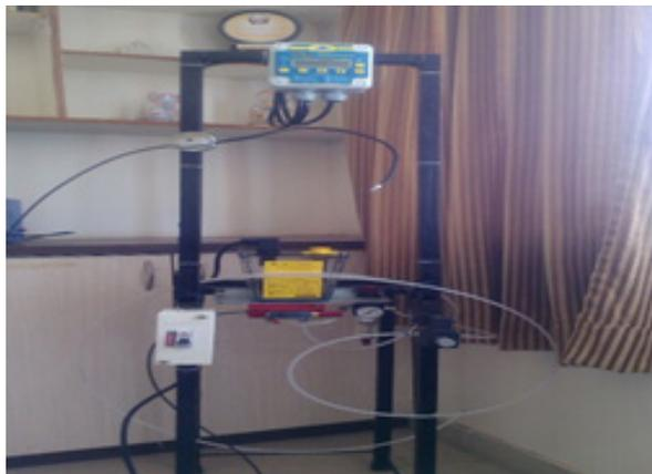
**Figure 2.** MQL fluid delivery Device.
