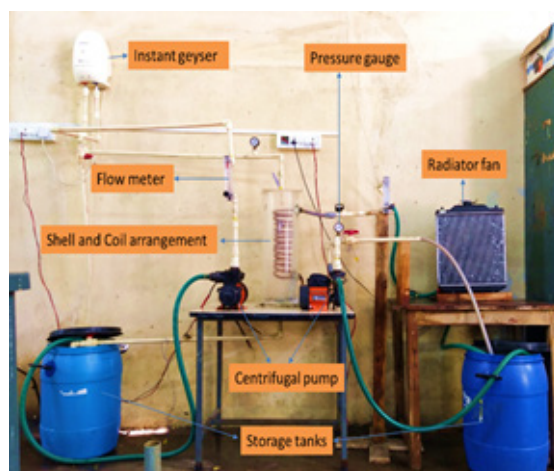
Figure 1. Photographic view of shell and helical coil tube heat exchanger.
