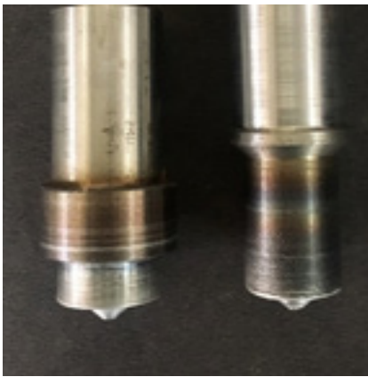
Figure 2. Tool used for welding.
