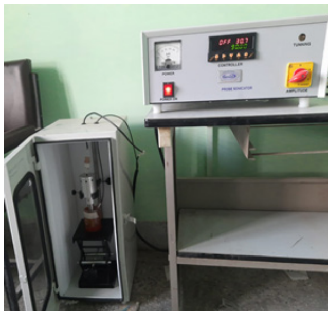
Figure 3. Fuel preparation by ultrasonic probe processor.
