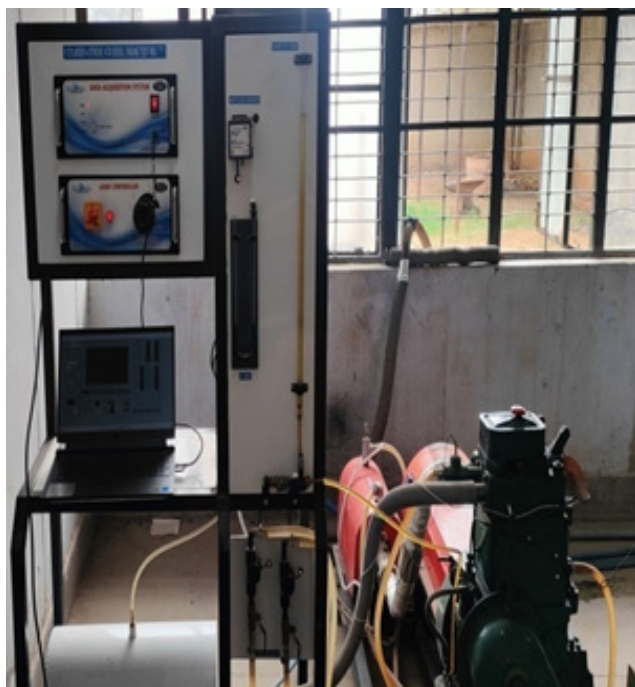
Figure 4. Engine setup for performance test.
