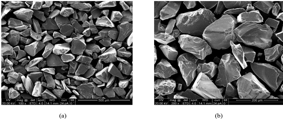
**Figure 1.** SEM of (a) 45 micron (b) 90 micron sized  $B_4C$  particles.
