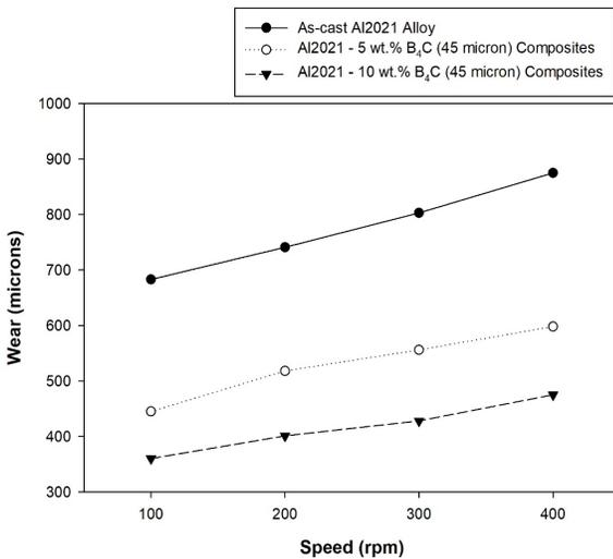
**Figure 10.** Wear of Al2021 with 45-micron-sized B<sub>4</sub>C composites at different speeds.
