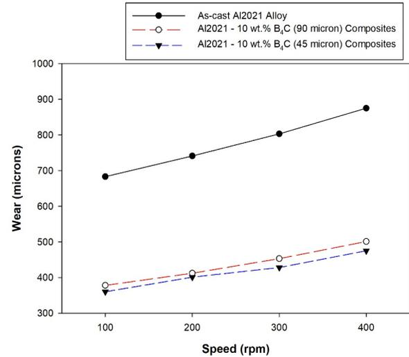
**Figure 11.** Comparison of wear of Al2021 with 90 and 45-micron B<sub>4</sub>C composites at different speeds.
