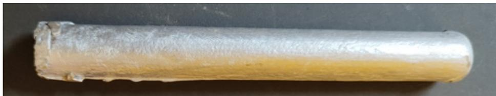
**Figure 2.** Al2021 alloy with  $B_4C$  composite.
