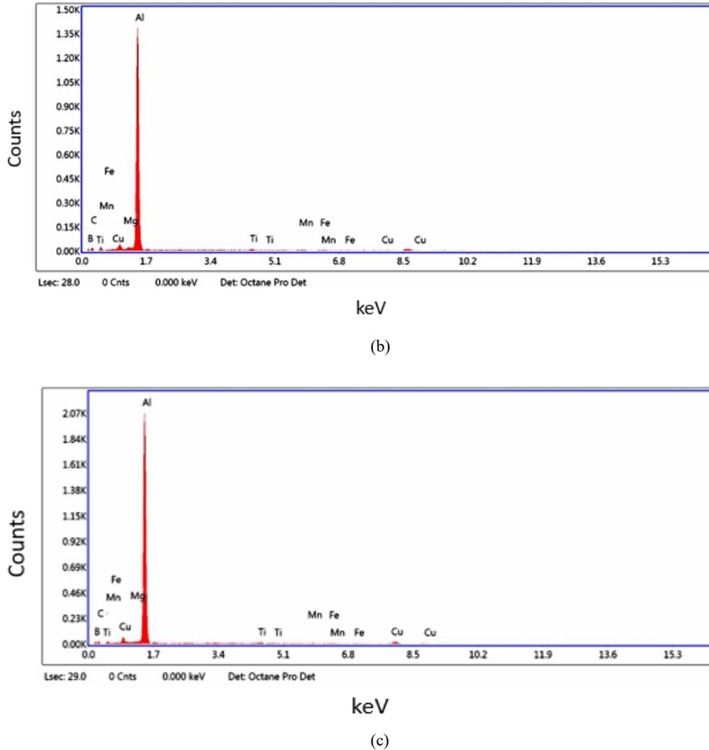
**Figure 5.** (a-c). EDS spectrums of (a) Al2021 alloy (b) Al2021 - 10wt.% of 90 micron  $B_4C$  composites (c) Al2021 -10 wt.% of 45 micron  $B_4C$  composites.
