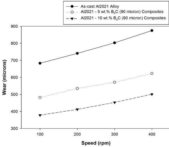
**Figure 9.** Wear of Al2021 with 90-micron B<sub>4</sub>C composites at different speeds.
