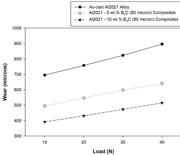
**Figure 6.** Wear of Al2021 with 90-micron-sized B<sub>4</sub>C composites at varying loads.
