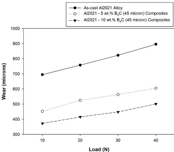
**Figure 7.** Wear of Al2021 with 45-micron-sized B<sub>4</sub>C composites under different loads.
