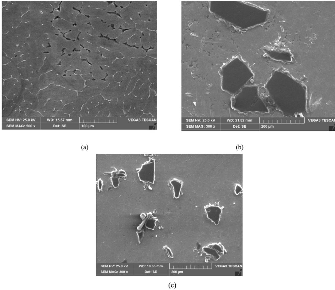
**Figure 4.** (a-c). SEM micrographs of (a) as cast Al<sub>2021</sub> (b) Al<sub>2021</sub> - 10wt.% of 90 micron B<sub>4</sub>C (c) Al<sub>2021</sub>-10wt.% of 45-micron B<sub>4</sub>C composites.
