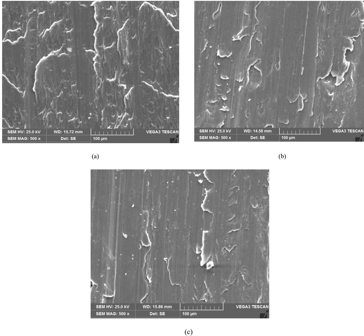
**Figure 12.** (a-d). Worn surfaces of (a) Al2021 alloy (b) Al2021 -10 wt.% of 90 micron  $B_4C$  composite (c) Al2021-10 wt.% of 45-micron  $B_4C$  composite.
