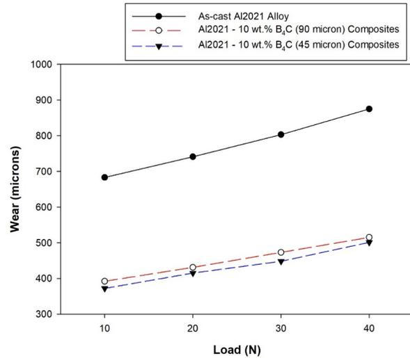
**Figure 8.** Comparison of wear of Al2021 with 90 and 45-micron-sized B<sub>4</sub>C at different loads.
