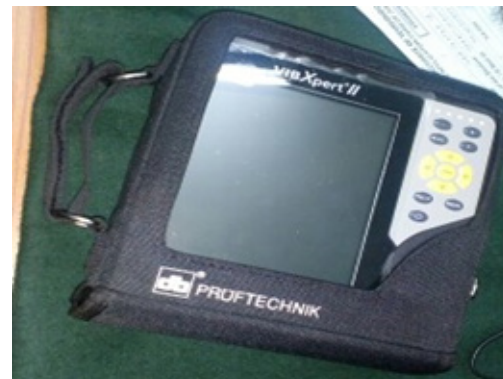
Figure 1. Vibrometer instrument along with measurement cables.
