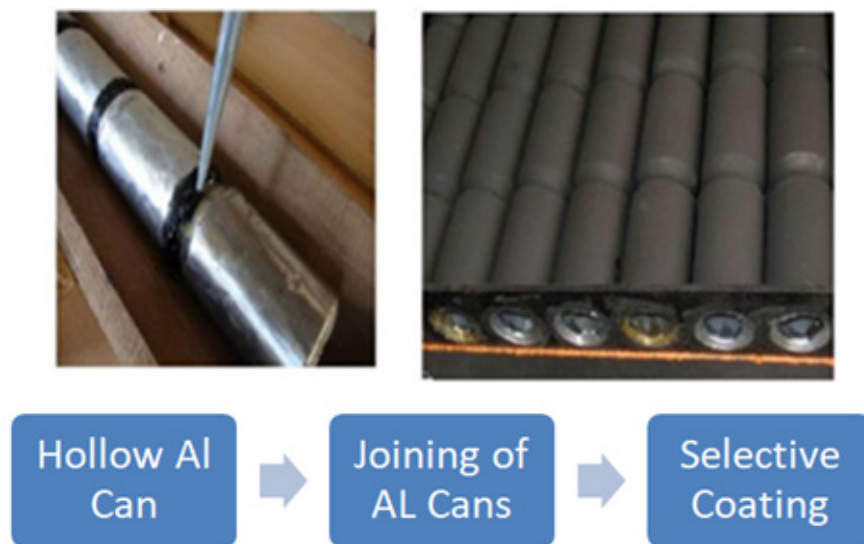
Figure 1. Solar collectors by using waste cans.
