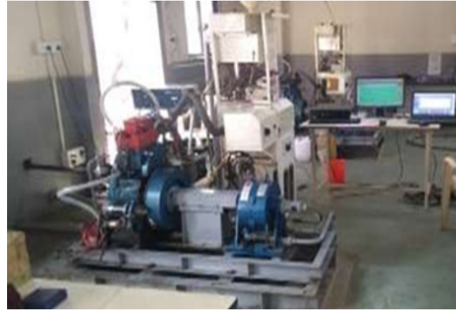
Figure 1. Computerized 4s, 1cyl, VCR Petrol engine test rig Source: Apex Innovations. (IC engine research lab).
