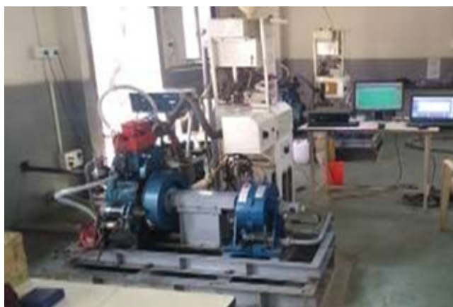
Figure 1. Computerized 4s, 1cyl, VCR Petrol engine setup Source: Apex Innovations. (Combustion research lab).
