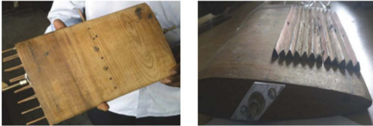
Figure 9. Smooth aerofoil profile and triangular roughness profile 11 .
