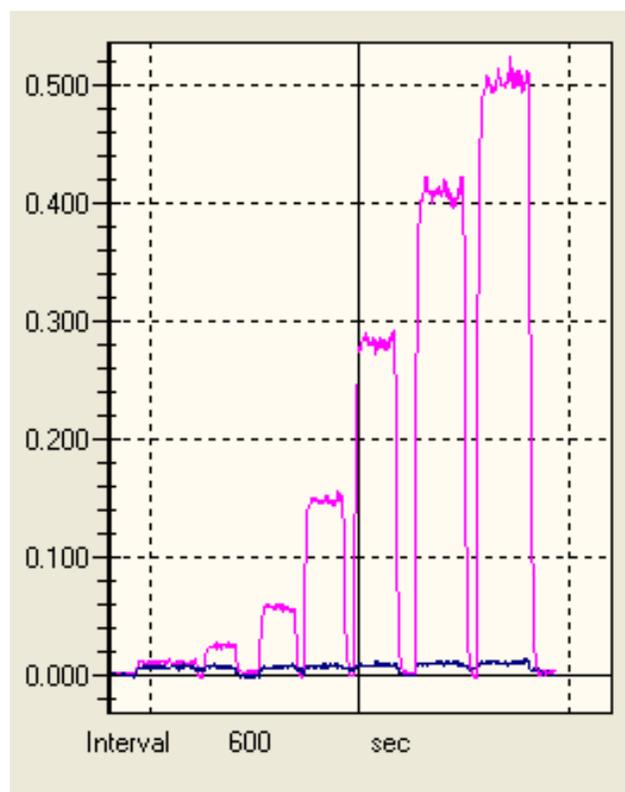
**Figure 3.** Linearity of Calcium standard.
