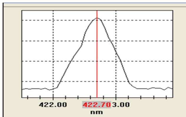
Figure 1. Calcium  $\lambda_{\text{max}}$  at 422.7nm.
