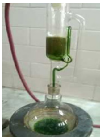
Figure 1. Extraction of Thymus vulgaris L. by Soxhlet apparatus.
