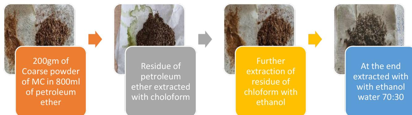
**Figure 2.** Schematic illustration of collection of extractive residues.
