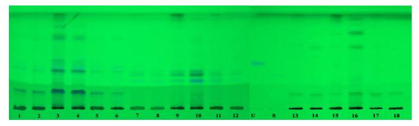
Fig. 4. TLC profiling of different extracts of A. marmelos. (254 nm).
