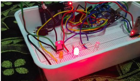
**IMAGE 1.** Red LED glows indicating that the system is locked.
