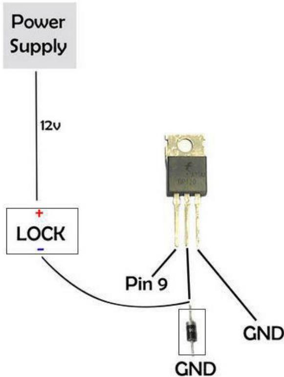
**Figure 3.** Connections to the Transistor TIP122.
