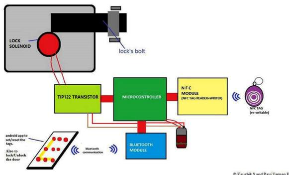
Figure 2. High Level Design of the Developed Lock.
